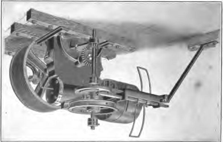
Fig. 40. Typical Ceiling Type of Worm-Gear Belt Elevator with Plate-Cam Belt Shipper
